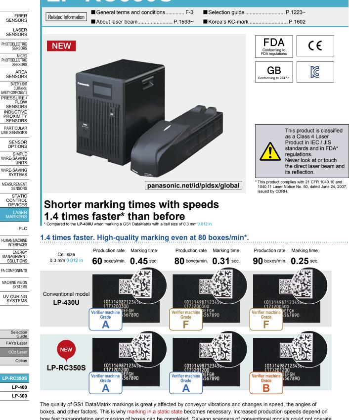
how fast transportation and marking of boxes can be completed. Galvano scanners of conventional models could not operate well at high speeds, forcing equipment operators to choose between speed or quality.
